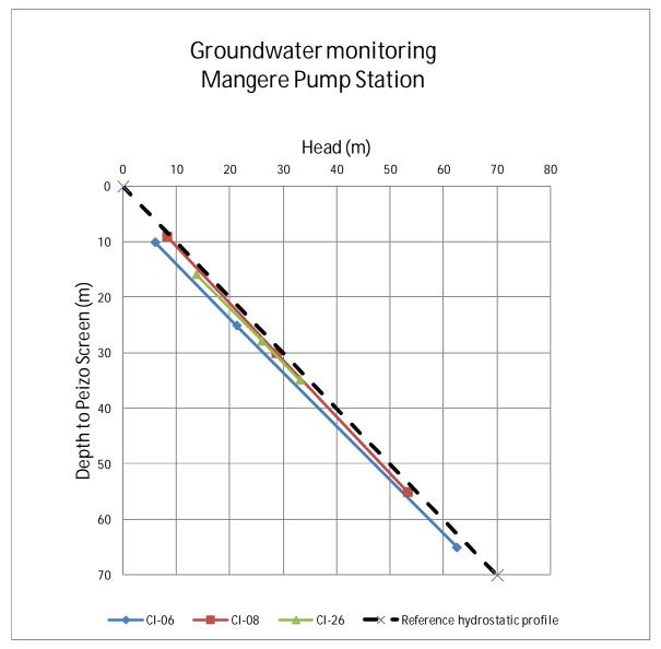
Figure 4 – Groundwater Levels from CI borehole piezometers, Mangere Pump Station, (MWWTP)
