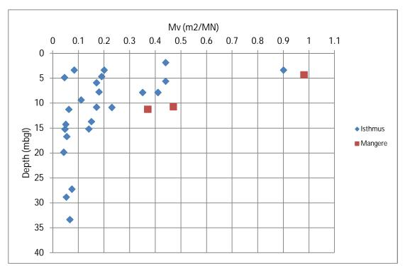
Figure 6 Mv for selected stress range (initial effective stress plus 50kPa)
