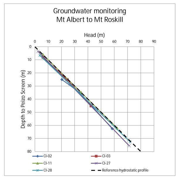
Figure 3 – Groundwater levels from CI borehole piezometers, Mt Albert to Mt Roskill
