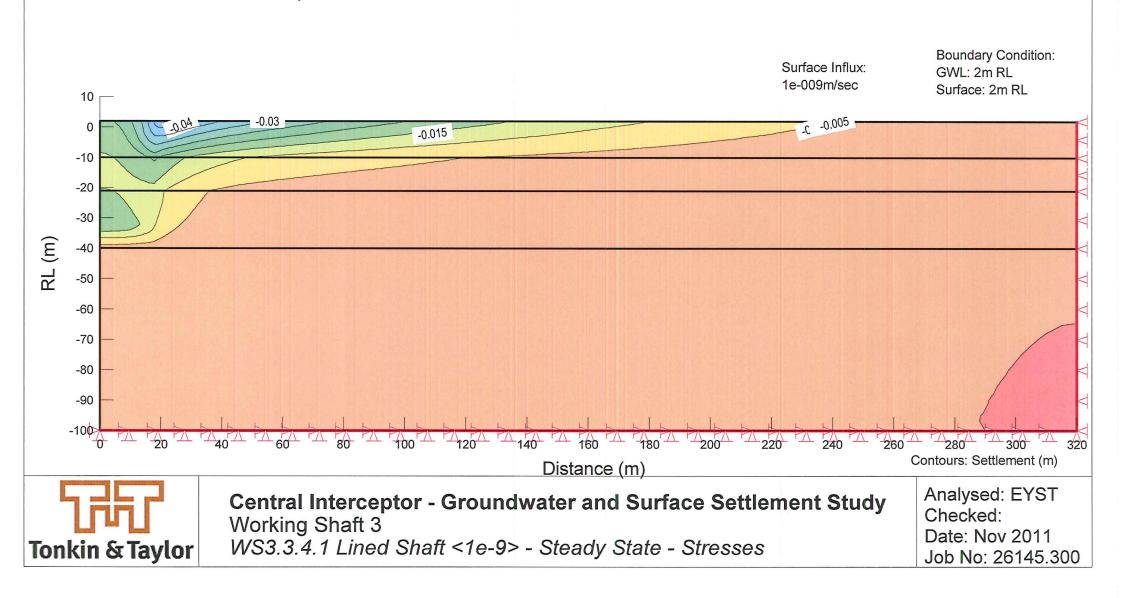
File Name: CI.GWS.AS3 axi.gsz Type: SEEP/W Analysis Method: Steady-State Scale: 1:1250 Analysis View: Axisymmetric Last Saved: 1/12/2011 6:10:34 p.m.
