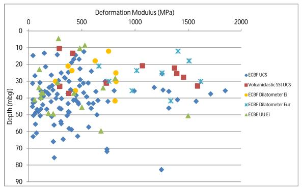
Figure 7 Deformation Moduli, Various Sources - ECBF Rock
