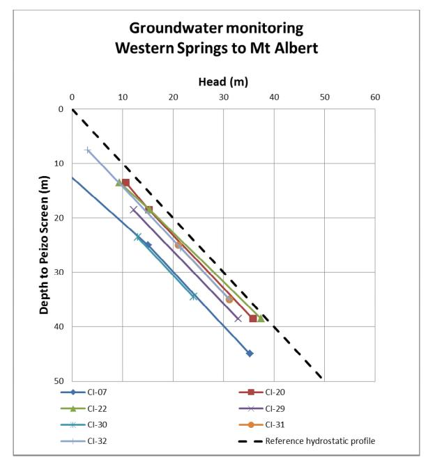
Figure 2 – Groundwater levels from CI borehole piezometers, Western Springs to Mt Albert Road
